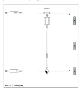
Should the maximum allowed lateral deflection of 4° be exceeded by determining the installation height, the program issues a warning.
